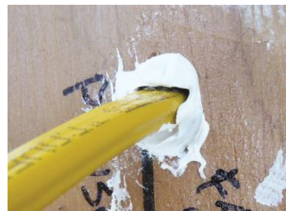
Figure 3. Caulks that failed the wire-movement tests typically remained bonded to the plywood but separated visibly from the outer sheathing of the cable.
