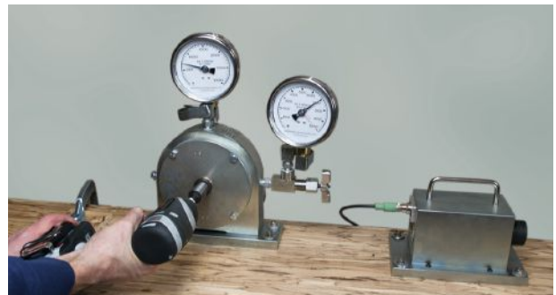
Tools were operated for three seconds while connected to a bolt tension calibrator. Results were displayed on a gauge in pounds of force, which were converted into inch-pounds with a digital torque wrench.
