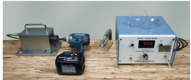
The meter converted average peak impulse into dynamic torque and displayed that value on a digital readout.
