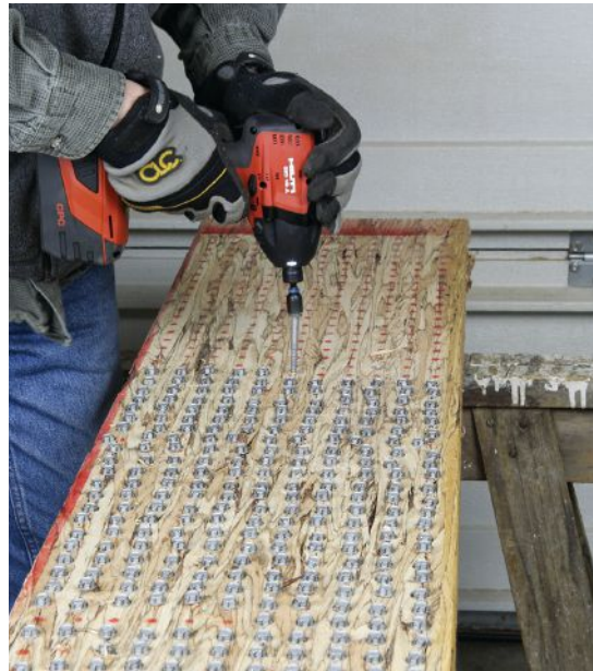
Runtime and speed were tested by driving 1/4-inch by 3 1/2-inch lags into a thick Parallam beam. The author counted the number of lags driven per charge and timed driving speeds.
