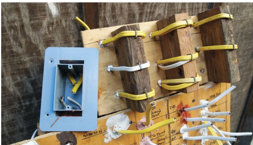
Figure 2. To evaluate the air-sealing effectiveness of two tapes and 22 caulks and sealants, the author applied multiple samples to test boards assembled from plywood, framing lumber, and sections of nonmetallic sheathed cable.
