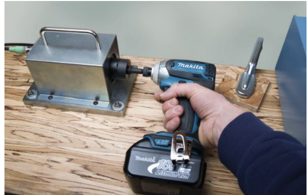
The author ran each tool for three seconds while it was connected to a digital torque tester cabled to a meter.
