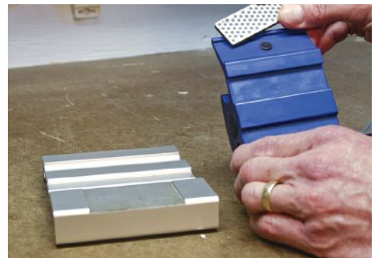
Powerful magnets anchor the interchangeable diamond stones to the wings of the carriage.
