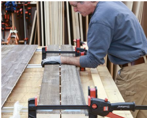
Figure 2. The author glued up the panels from shiplap siding, ripping the edge profile off glue joints and reinforcing them with Festool Domino tenons (left). Squeeze clamps pulled the glue-up tight to the bar clamps and helped keep the panels flat (below).
