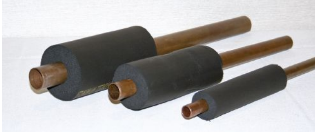
Figure 4. Pipe insulation prevents heat loss and improves system performance, especially when pipes are located underground or outside the thermal envelope. Wall thickness of the insulation should at least equal the nominal diameter of the pipe.
