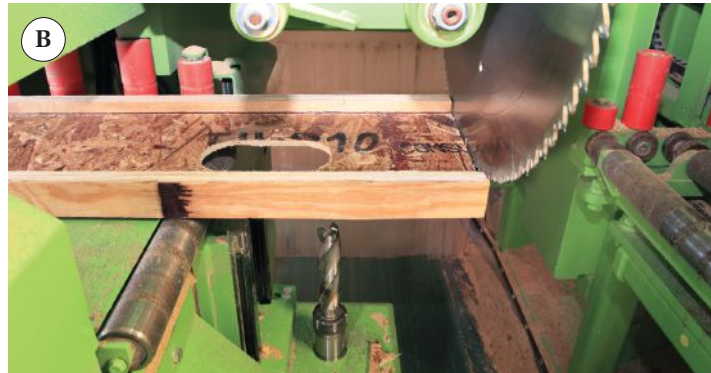
Figure 2. The engineered framing stock is cut with CNC equipment that can accurately trim I-joists and LVLs to length and cut bevels (A). The machine can also cut rafter-tail profiles and make hvac cutouts (B, C).
