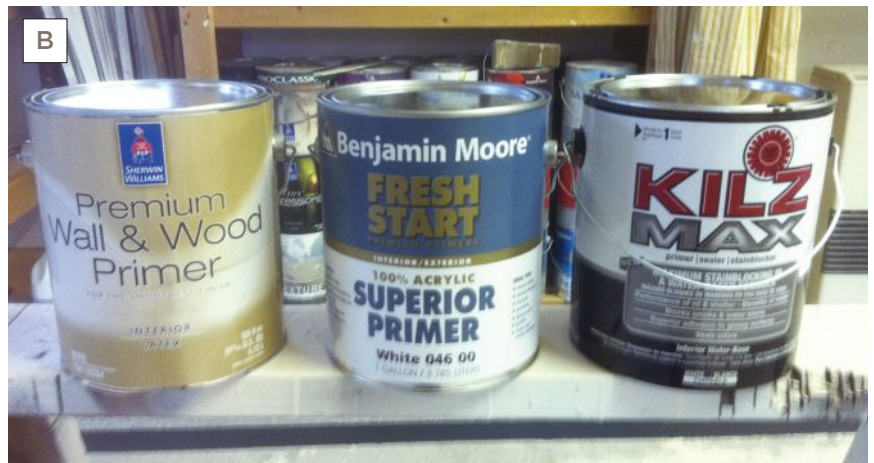
Figure 2. After patching nail holes and dings and sanding again, the author primes the trim (A) with a fast-drying sandable waterborne primer (B). Waterborne primers raise the grain, so once the primer has dried, he sands it with 150- to 180-grit paper to smooth out the surface and prepare it for top-coating (C).
