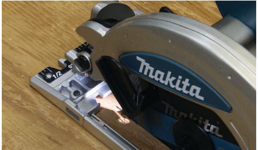
The Makita saw has a built-in light that is activated when the trigger is depressed slightly; the Hitachi and Ridgid are similarly equipped.
