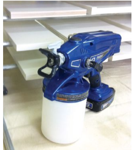
Figure 4. Graco's ProShot 18-volt cordless sprayer works well with waterborne primers and paints and is easy to clean afterward. It holds just a quart, though, so the author reserves it for smaller jobs.
