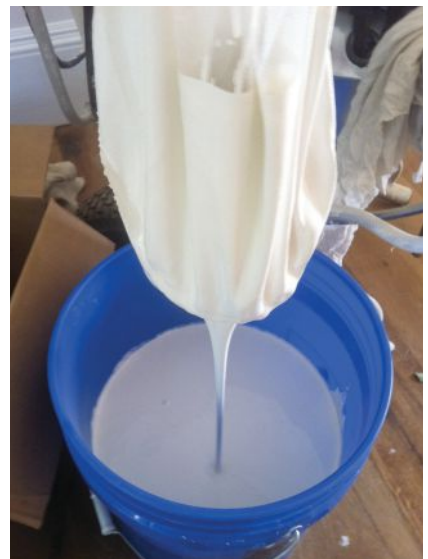
Figure 5. Whether brushing, spraying, or rolling, the author strains all waterbornes — even freshly opened gallons — before using them.
