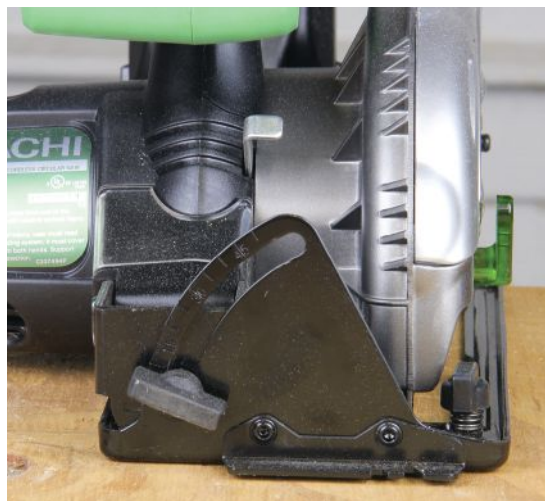
Contrasting colors and graduations one degree apart make the quadrant on the saw above easier to set and read than the quadrant on the more basic model at left.
