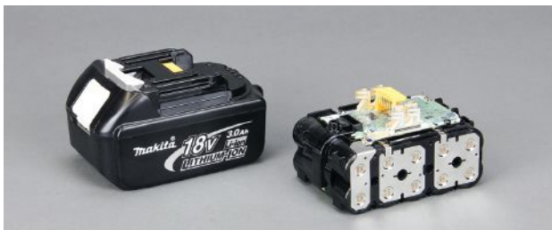
Like other full-size 18-volt packs, the Makita LXT battery has 10 cells.
