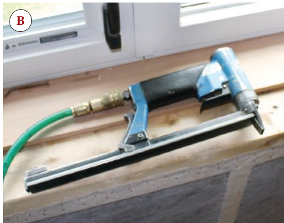
Figure 2. To minimize bulging of the cellulose between framing members, netting is stretched tight and fastened with a pneumatic upholstery stapler (A, B). The closely spaced fasteners are driven at an angle just beyond the outer edges of the faces of framing members. This “inset stapling” helps draw the material taut and prevents the cellulose from pushing beyond the framing (C). The tension of the netting against electrical boxes is enough to prevent them from filling with insulation when the cavities are packed; the netting will later be cut by the drywall crew (D).
