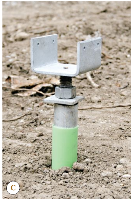
Figure 1. Helical piers have a screw-shaped plate welded to a zinc-coated steel shaft, and are made in different sizes for different soils and applications (A). As the driver turns the pile, it simply screws into the ground until the installer is confident it's below the frostline and in soil with sufficient bearing capacity (B). Several types of caps are available to attach piers to framing; some are adjustable in order to fine-tune the elevation (C).
