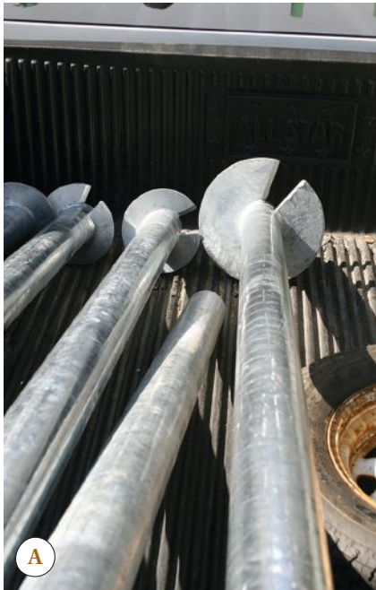
Figure 1. Helical piers have a screw-shaped plate welded to a zinc-coated steel shaft, and are made in different sizes for different soils and applications (A). As the driver turns the pile, it simply screws into the ground until the installer is confident it's below the frostline and in soil with sufficient bearing capacity (B). Several types of caps are available to attach piers to framing; some are adjustable in order to fine-tune the elevation (C).
