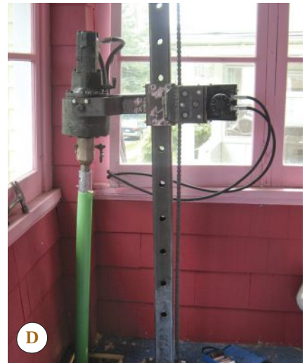
Figure 6. The author's small rig excels at going places larger pile-driving equipment can't (A, B, C). When the machine won't fit into a tight area, the drive head can be mounted on a portable bracket that bolts to the structure (D).
