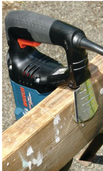
The fold-out hook is deep enough to grab a 2-by or an extension-ladder rung.
