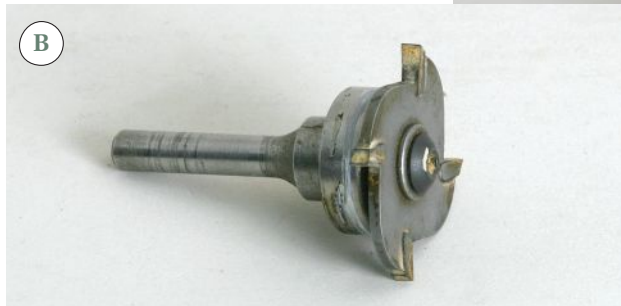
Figure 2. After years of weatherstripping old windows and doors, the author has settled on three seal profiles for most jobs: a polypropylene brush seal for the sides; a 1/4-inch tube seal (white or bronze) for the meeting rail, and a white 3/16-inch tube for the bottom (A). Slots for the seals are cut with a 3-millimeter slot cutter (B); the seals are installed with a screen tool or by hand (C).
