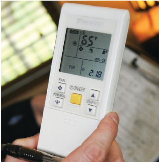
Figure 3. Unlike most hvac equipment, which cycles on and off as a thermostat calls for heating or cooling, inverter-driven ductless heat pumps ordinarily run continuously, adjusting their output as needed to maintain a constant indoor temperature. A remote supplied with each indoor unit controls temperature, blower speed, and the position of the vent louvers.
