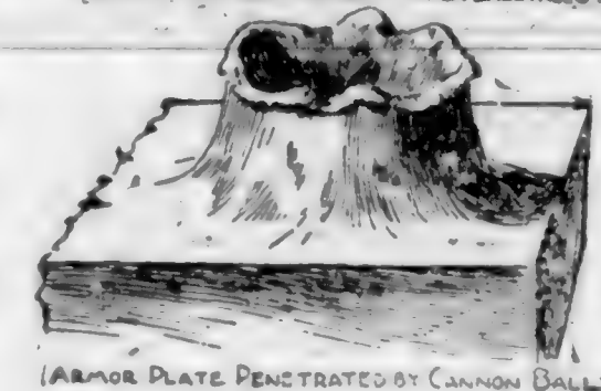
ARMOR PLATE PENETRATED BY CANNON BALL.
