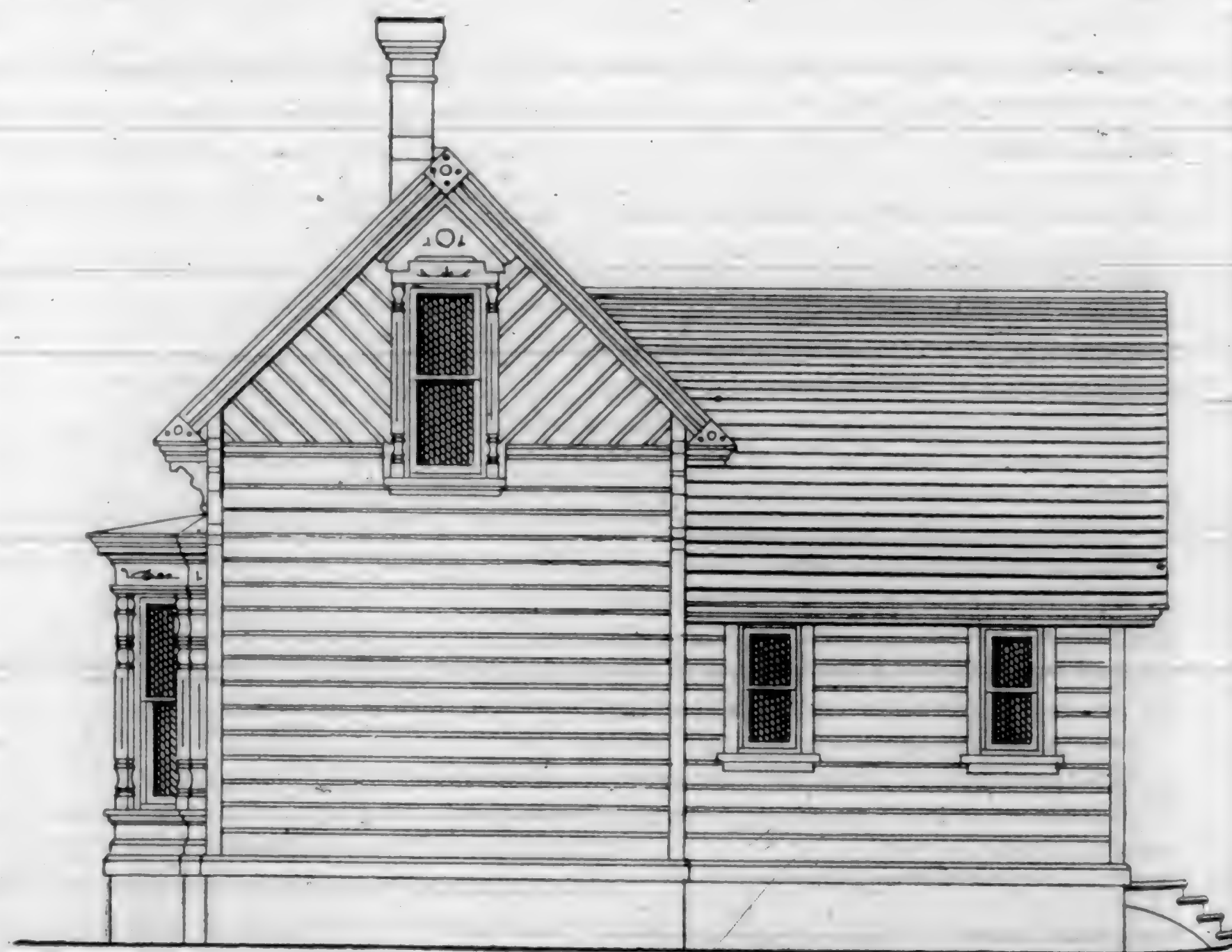
PLATE 5.—SIDE ELEVATION OF WORKINGMAN'S COTTAGE.
