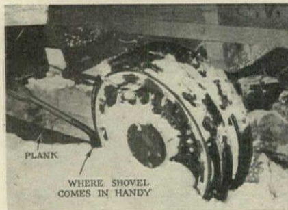
A shovel will often get a truck out of a snowbank when nothing else will do. Below—Motor trucks enable the steam shovel to deliver full capacity
