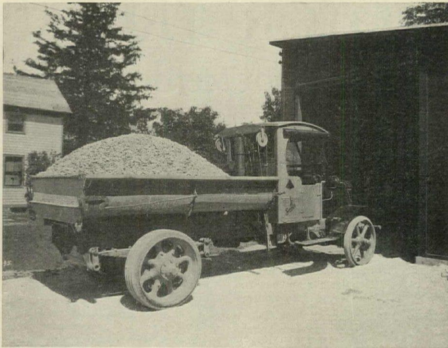
It is not well to overload the truck. Note how flat the rear springs are
