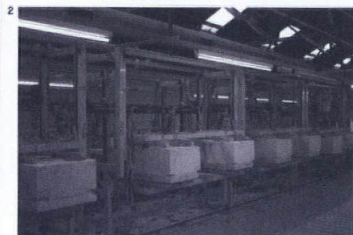
1. Clay slip being poured into a plaster mould, the plaster column helps to build a head of pressure 2. The Belfast sink casting hall, where heavy plaster moulds are held and mechanically manipulated
