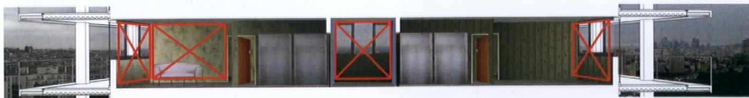
addition of new elements and demolition of partition walls
