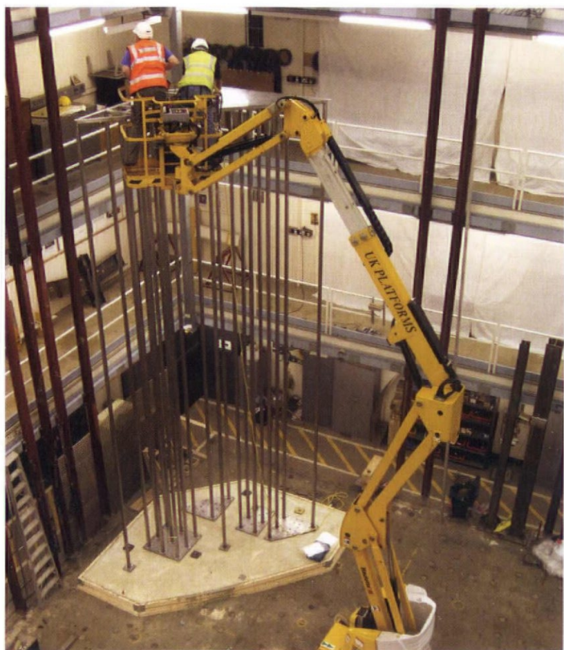
Left_ A stockpile of dampers, showing cable suspension Below_ The Building Research Establishment at Watford, one of many test rigs for the pavilion
