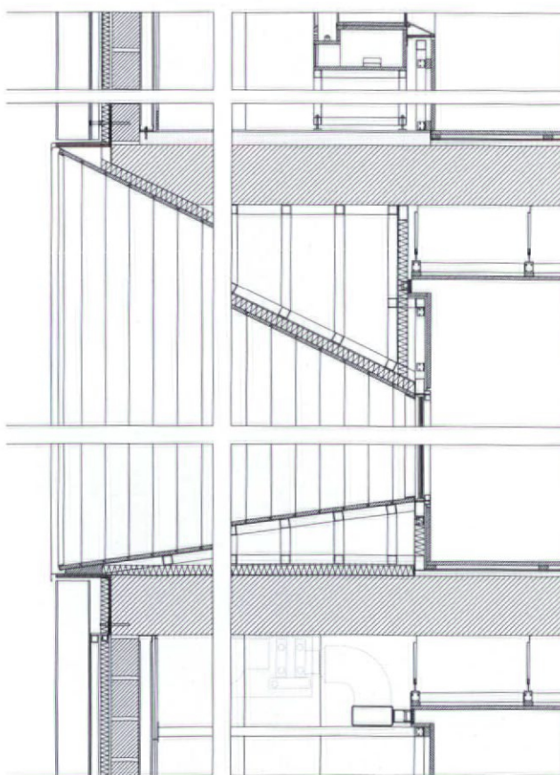
detailed section through external wall and window reveal
