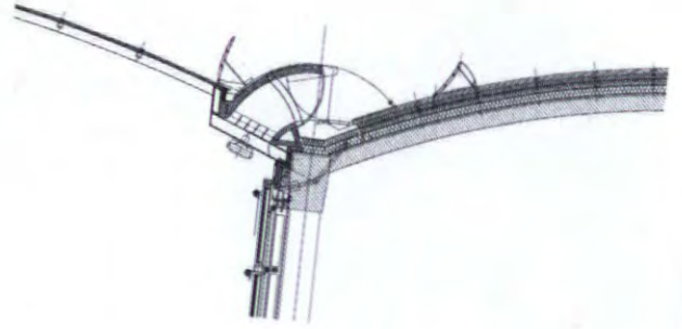
detail of court and office roof junction
