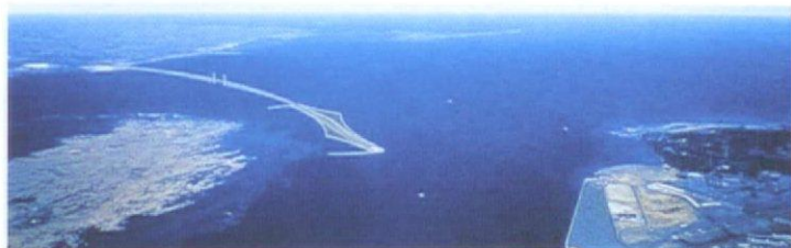
1 Øresund link from north with Saltsjöholm island in foreground; bridge and Swedish coast to left; tunnel and artificial peninsula off Amager on right.
