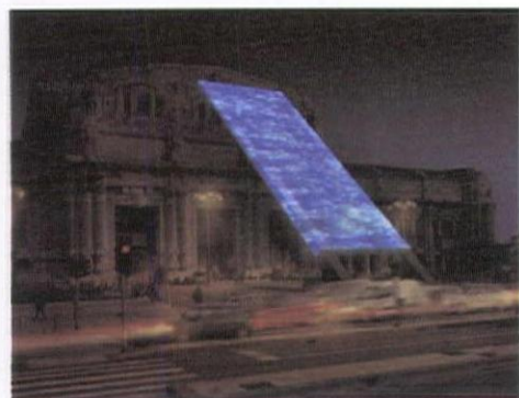
Ian Ritchie's winning design for a light installation in Milan; two tubes support a sparkling web of fibre optic cables.
