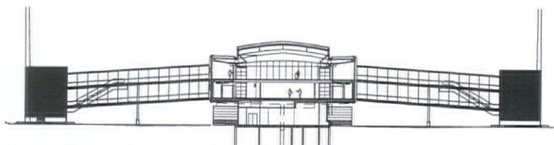
cross section through pier and air bridges
