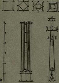
2, stages in the design of a pinnacle according to Roriczer.
