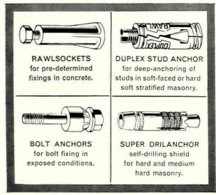
Rawlbolts are the world's finest bolt-fixing method. Quickly and easily applied, the resultant anchorage in good quality masonry is stronger than the bolt. Used in their millions, Rawlbolts are only one of the Rawlplug Range of bolt, cavity and screw fixing devices. Other members of the fantastic bolt-fixing group are shown in the box.
