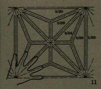
11, Redrigo Gil de Hontanon's rule for the section depths of the ribs of a late Gothic vault in terms of the mean bay width 'b', these depths being notionally scaled in proportion to the outstretched thumb and fingers of the hand.
