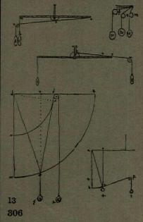
modern principle of virtual work and opened the way to a quantitative study of simple machines and their mechanical advantages. The second, with its Euclidean basis and tight Euclidean logical structure, was rigorously quantitative throughout and first introduced the concept of the centre of gravity and furnished the means for calculating its position.
