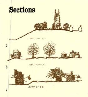
the street with, at the west end (B-B), the northern pavement considerably lower than the road and the grass verge sloping up between them (see also 2). C-C shows the section at the widest point and D-D at the centre of the town where the ground now rises slightly to the north (i.e. the church is built at the highest point of the town), then falls steeply to the railway below.
