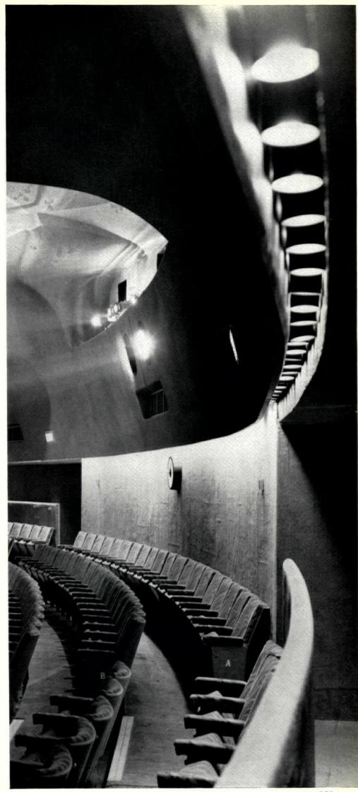
In the subdued blue lighting (blue because it was found that white lighting killed the blue in the carpet) the staircase treads, each with a masked strip light, float airily and contrast with the solid black handrails. (The lights under the bottom treads should, however, be removed, as the additional thickness of carpet cuts out all but a few chinks.)
