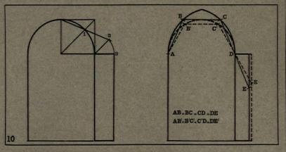
10, two geometric constructions to determine the size of buttress needed by a given vault; that on the left according to Rodrigo Gil de Hontanon, and that on the right Blondel's rule.
