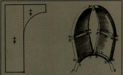
14, above left: the basis of Wren's static analysis of the size of buttress needed by a given vault. Above right: the mode of collapse of the dome of St. Peter's visualized by the three mathematicians. Below: an identical mode of collapse (smaller sketch) and a converse one in which each rotation takes also in the omesite sense (larger sketch) as visualized by Teonardo.
