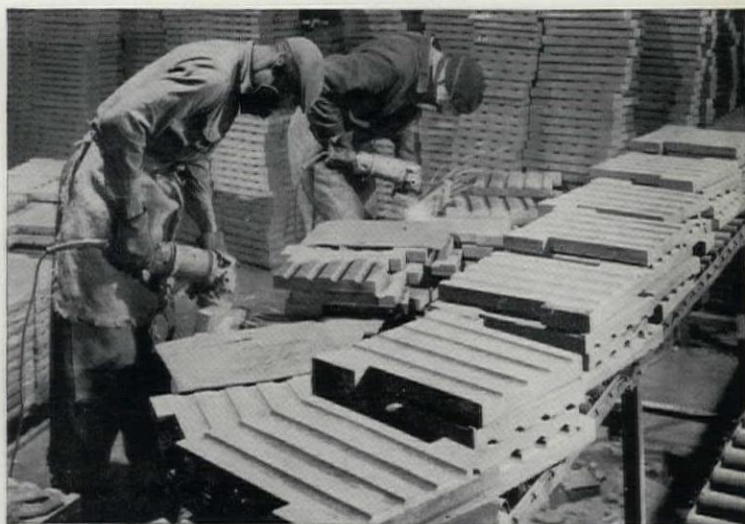
The cast-iron storage core blocks are produced in the T.I. Group foundry at Oldbury—to ensure the finest possible quality and reliable delivery times.
