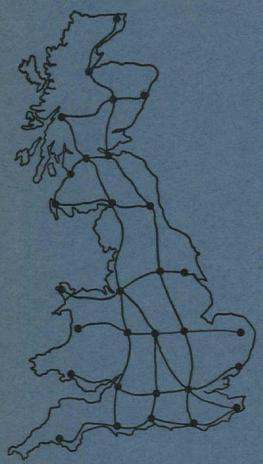
Diagram 2: possible network for 250 m.p.h. operation; stations are marked only at intersections or terminals. Other stations or regional feeder networks could be added were appropriate.
