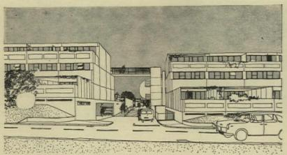
The approach from the access road, showing ramp down to car parking beneath terraces and ramp up to service road, with nedestrian bridge linking terrace decks
