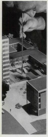
9, 'Modelscope' in use. The viewing lens at base of the tube provides a true ground level perspective.
