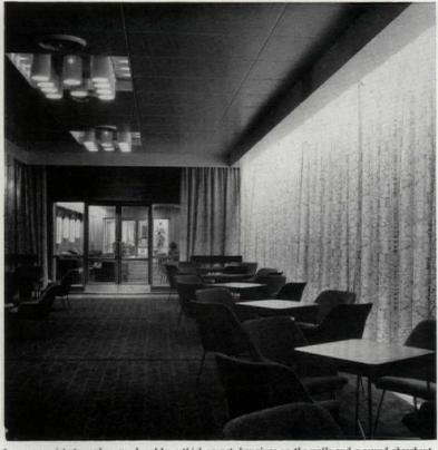
1, a very quiet atmosphere produced by a thick carpet, hangings on the walls and a sound-absorbent ceiling. (Ballroom in the P & O and Orient Line steamship Orsova; architects, George, Trew & Dunn.) 2, honeycomb brickwork for sound absorbent treatment. (End wall of the gymnasium-hall of a school in Staffordshire; architects, Andrew Renton & Associates.)
