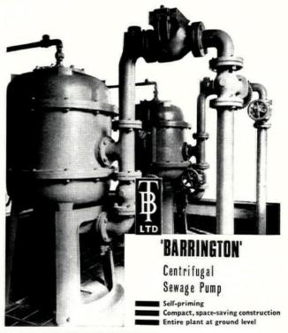
The simple and efficient self-priming system, together with the robust construction of all components with all working parts at ground level, makes the "Barrington" the most outstanding development in centrifugal sewage pumps in recent years. Available in a range of sizes for discharge rates from 50 to 1,000 g.p.m.Illustration shows two 3"pumps installed at Partridge Green for Horsham RDC. Consulting Engineers: Howard Humphreys & Sons
