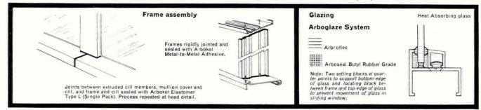
In the Merrion Centre, Leeds, the Arboglaze system incorporated: Arbomast B.R. high polymer adhesive sealant for joint caulking and weather sealing.
