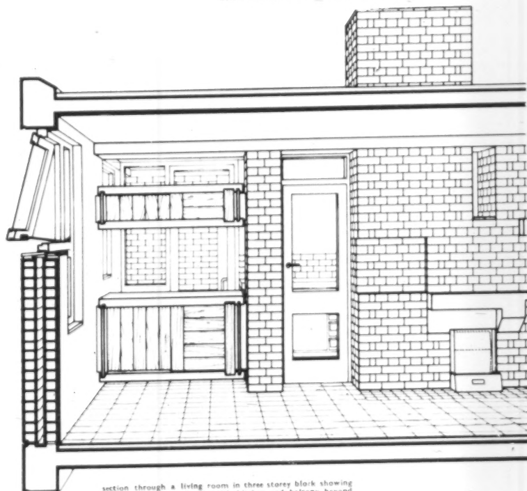
section through a living room in three storey block showing fireplace and serving unit with kitchen and balcony beyond
