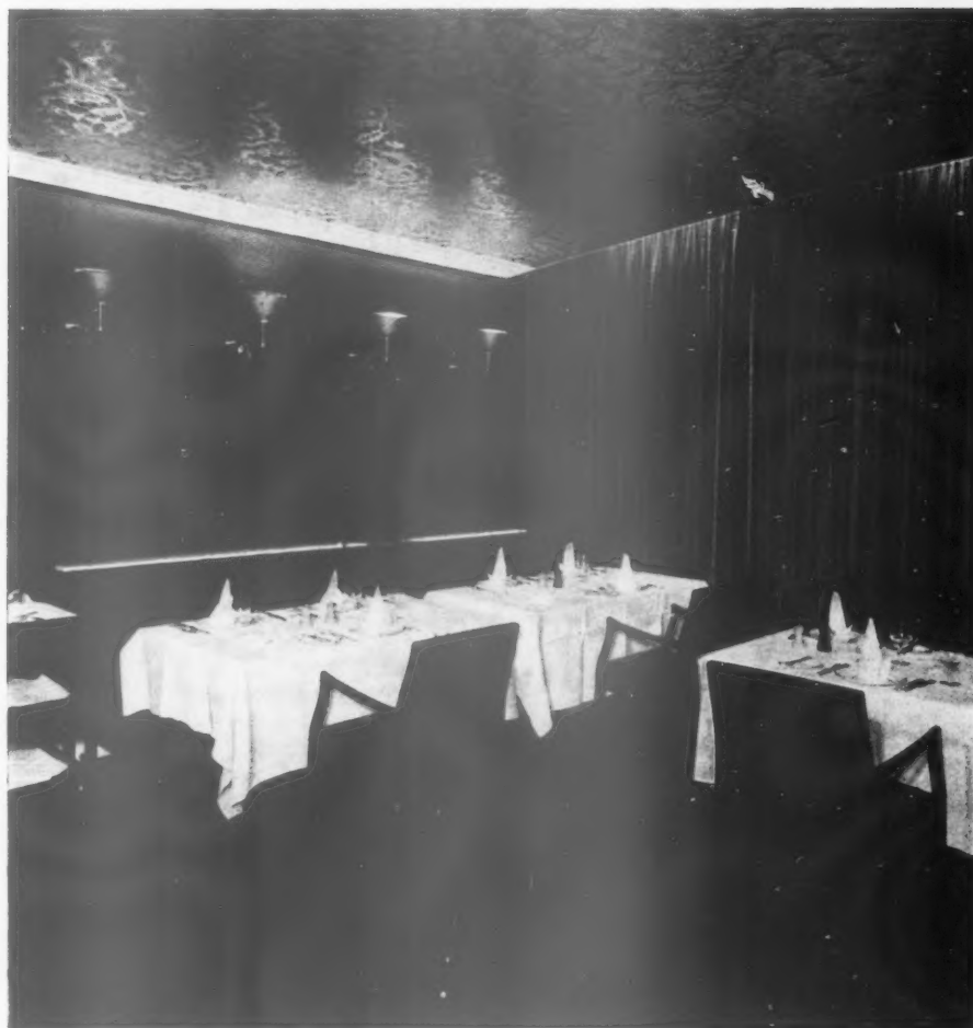
1, corner of the restaurant immediately to the left of the entrance from the foyer. At the edge of the gold papered ceiling are white louvers above which is concealed lighting and ventilation.
