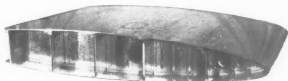
14, a sandwich skin wing of Handley Page design. Stiffness is obtained by the corrugated-core sandwich skins and webs. The multiple spars provide a measure of reserve strength in the event of a failure in flight. This type is analogous to 13 but is for lighter loading, as in transport aircraft. Fuel would be carried between the webs.
