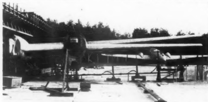
32. structural testing of the Bristol Britannia at Farnborough. The double exposure shows the amplitude of the working deflection. This particular test applies fluctuating wing loads to simulate the effect of gusts, while the fuselage pressure cabin is pressurized and released under water in the tank on the left, to represent the once-per-flight pressure loads. These tests are necessary because of the impossibility of predicting fatigue life reliably from theoretical considerations. (Crown copyright reserved.)
