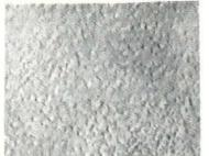
19, Heavy and light 'Stucco' rolled finish for aluminium roofings.
