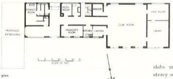
This club\* for the Haileybury Guild, in Ben Jonson Street, near St. Dunstan's Church, replaces a smaller one on the same site which was bombed. Load-bearing brickwork is used throughout, and the roofs are of timber joists, wood-wool
