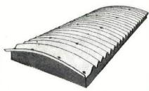
5. a continuous strip rooflight in corrugated 'Perspex.' Widths up to 8 ft. without extra support are possible.
