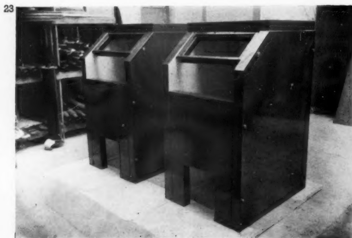
23, covers for riveting machines comprising a core of glass silk with perforated metal on the inside and sheet metal outside, manufactured by Burgess Products. 24, sprayed Limpet asbestos fibre.
