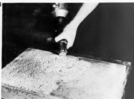
Bush-hammering a Cornish granite slab.
