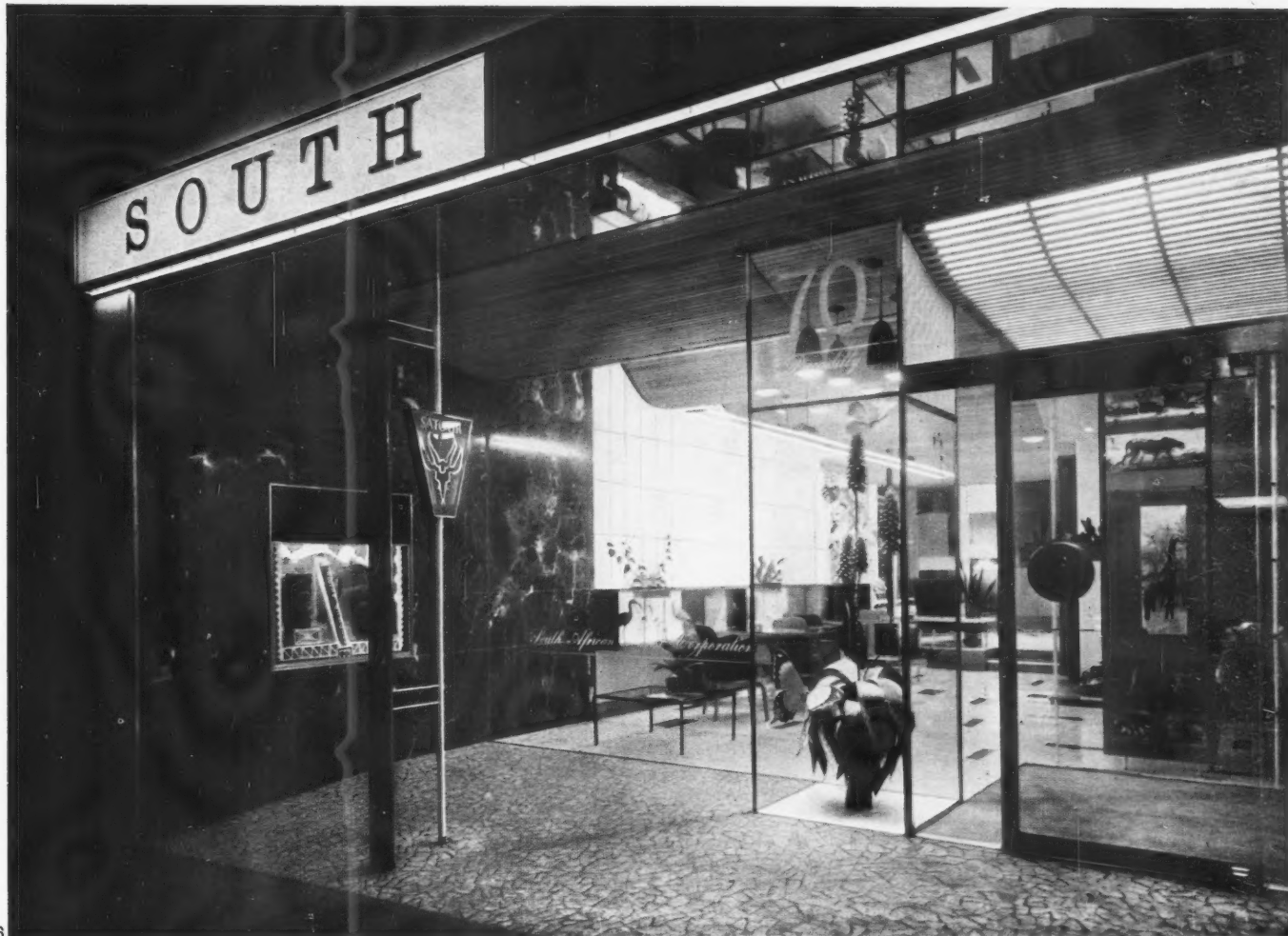
The main façade showing the set-back of frameless plate glass and the Tinos marble wall panel which continues into the interior. This is the most advanced and imaginative example of the disappearing shop front to be carried out in London to date.
