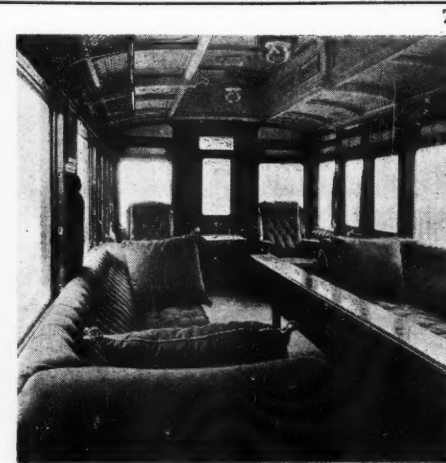
7, G.W.R. family saloon of the same period. Upholstery is in peacock blue broad-cloth with gold lace. Note the clerestory roof and the large amount of window space, a characteristic feature which has not been improved upon even in the latest all-steel coaches.
