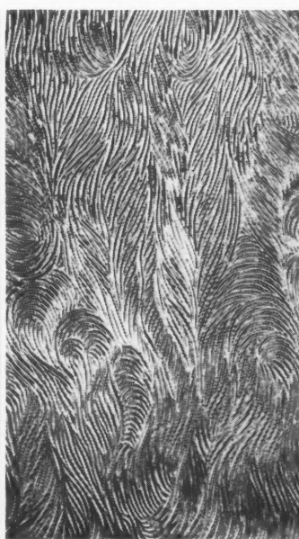
MERSEY Of the non-formal group. Average diffuse light transmission 80%. Diffusion and obscuration values approximate to \frac{1}{8} " Rolled Glass. Degree of obscuration is greatly influenced by the direction of glazing.
