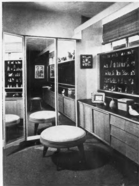
Top right, principal bedroom. Continuous radiator under window. Bedback of straw matting; bedspread of red handwoven fabric. Centre and bottom right, the dressing-room. All woodwork natural oak. Wall cabinet has sliding fibre-board doors. Wash basin is set flush in the black linoleum counter. Carpet natural felt.
