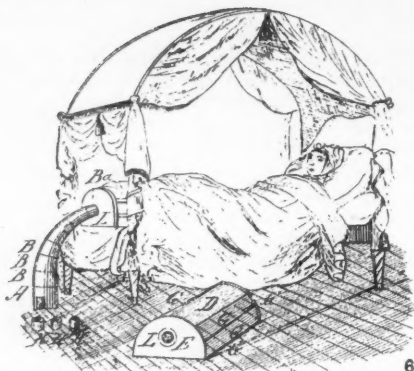
6, American Steam-Bed Bath, 1814. The steam bath was regarded primarily as a medical treatment in the early nineteenth century—hence its frequent association with beds. Everywhere, from the beginning to the end of the century, apparatus generating steam in more or less complicated ways were invented. (U.S. Patent 2049x, 21 January 1814).
