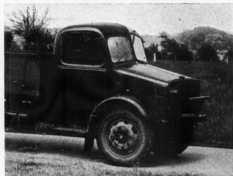
4, more sturdy-looking than stylish, this war-time Bedford truck, with its broad bonnet sloping up to meet the one-piece cab of pressed steel, breaks away from the traditional nose-shape. Vehicles of this kind may well help to accustom the public to the short down-curving radiators which neither Chrysler nor Fiat succeeded in popularizing before the war.
