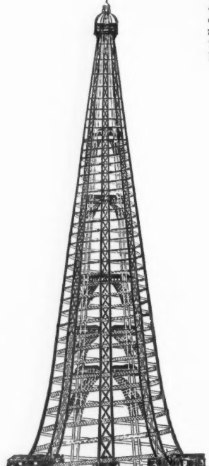
"The eight main ribs or vertical girders are formed of four cruciform shaped columns. A two-track spiral electric railway, gradient 1 in 6, would travel at 5 miles per hour, and 1,600 passengers per hour could be conveyed by it. There are six Bungalows on the 3rd stage and a Photographic room. On the 4th stage are four club-houses, to be let to London Clubs. On the 5th stage two large Dining or Reception Rooms to be let for private entertainments. On the 6th or top stage there are four look-out Bays, one Meteorological Room, Photographic Room, small Café, and a room for a siren Fog-horn to be used in conjunction with a Phonograph for advertising purposes. A powerful Electric Searchlight would be fixed in the Lantern, and a projector provided." By "Altiora Peto" (Henry Rose and E. J. Edwards, of London). 1,274 feet high. In steel framing, carrying tiles or terra-cotta panels.
