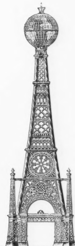
"The design is composed of a group of five Towers, a main central one supporting a large terrestrial globe, and four secondary ones. The great spaces, both inside and outside the Globe, will form the principal attractions to the Tower. The interior of the Sphere will be divided into several floors." By Lamont Young, of Naples. 1,450 feet high. In iron.
