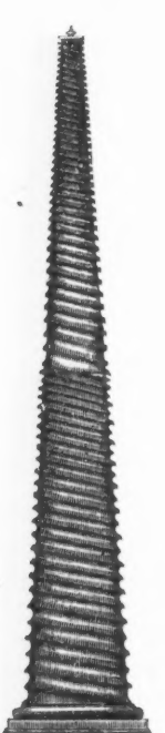
"The shell of the Tower to be constructed of corrugated steel with 60 corrugations. The corrugations to run in straight channels from the bottom to the top. The bottom plates to be 1 inch thick, with a radius of 4 feet 6 inches, and to taper to the top of the Tower to corrugations 9 inch radius of 3 inch plates. A Spiral Promenade from the bottom to the top is provided, also a Spiral Road for tramcars reaching only half-way up. A telescopic lift 150 feet long is intended to be used in calm weather, worked by hydraulic power." By J. Horton, of Halifax. 1,200 feet high. In corrugated steel.
