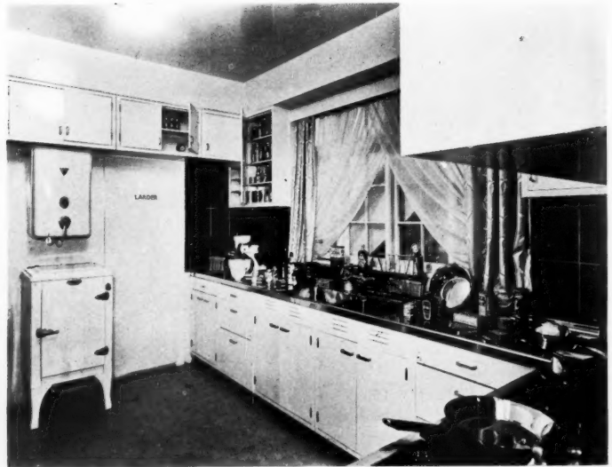
A kitchen equipped by Arundell Clarke with pressed-steel standard kitchen units. It will be noticed that an unbroken flush surface is given as though the units beneath the sink had been purpose-made to fit exactly into this particular kitchen. This is achieved by inserting special metal dividing strips between adjacent units.
