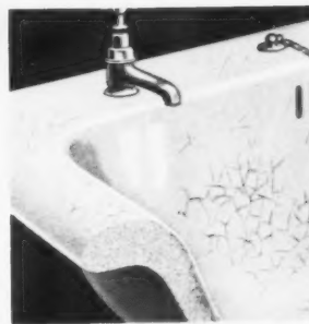
Ordinary ware showing crazed surface and fouled, porous body.
