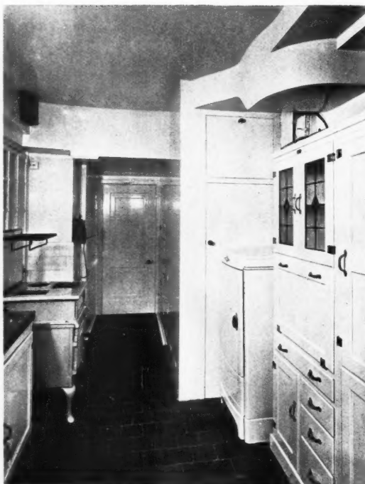
One of the kitchens at Eaton House. The air conditioning plant is housed in the insulated cupboard to the left of the refrigerator.
