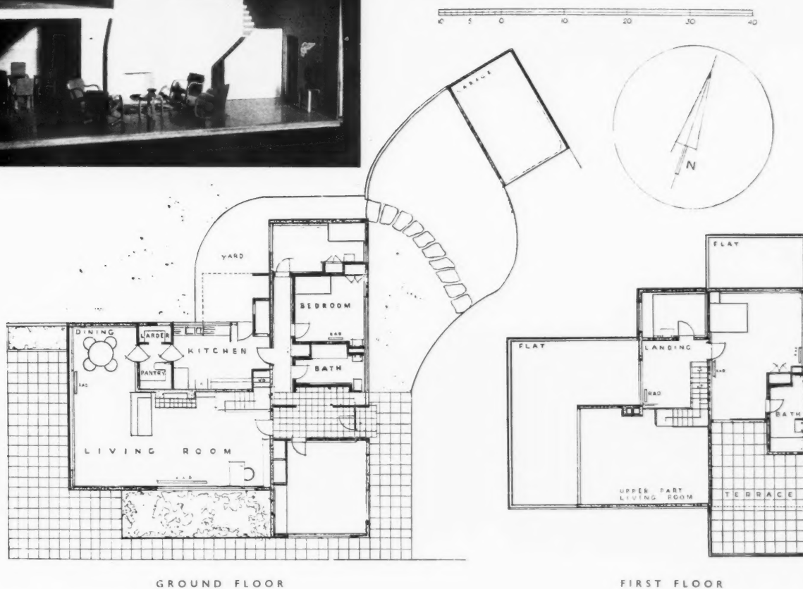
PART OF THE LIVING-ROOM is carried upwards through two floors, to a height of 18 ft. so that the staircase landing becomes a gallery overlooking the living space. The arrangement is shown clearly in the model, made by boys at Oundle School under the direction of Mr. Richard Finney.
