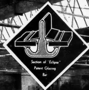
'ECLIPSE' PATENT ROOF GLAZING AT NEW PRINTING WORKS, EASTLEIGH
