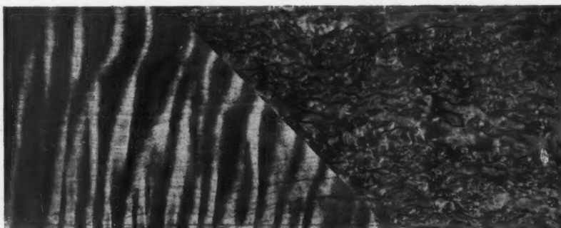
6. A contrast in birch-plywood veneers. Both halves of this sheet are of Finnish birch, the left being ordinary birch with a good streaky figure, and the right the rarer burr-mottled "Flame Birch" obtained from trees of the same species, growing in bogs.
