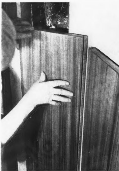
Finished material : three forms of faced plywood : 3, seven-ply cased on both sides with galvanized iron, 4 and 5, fitting panels together ; that in 4 being veneered with silky oak, and that in 5 faced with black bakelite.
