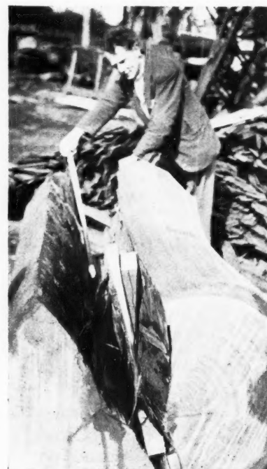
1. Cleaving oak for cleft oak fencing. See the complete process illustrated on the facing page.
