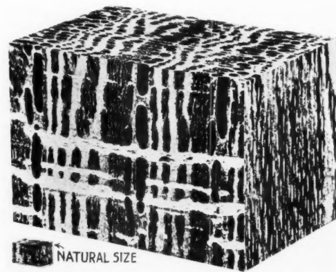
11. A model block of common elm magnified 8½ times to show the wood-structure in section.
