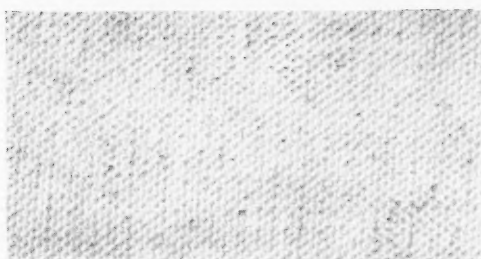
The texture of the canvas duck used for the external face. It takes paint admirably.
