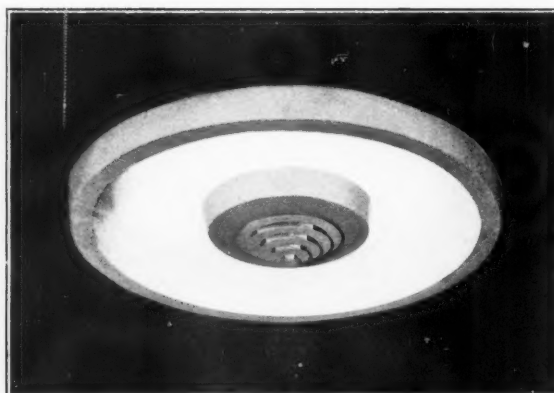
A Stylovent lighting and ventilation fitting, made in steel, brass, and other metals. The lighting is diffused from the boxel around the air diffuser. The function of this diffuser is instantly to distribute the high speed incoming air at the point of entry so that bulky expansion boxes can be dispensed with.
