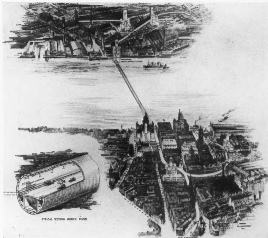
Top. A drawing showing the lay-out of the Tunnel across the river Mersey from Liverpool to Birkenhead, and the system of ventilation. Centre. The New Quay Ventilation Station, Liverpool. A large garage is attached to the building to accommodate the motor cleaning machine for the Tunnel, break-down and repair wagons. Bottom. A view inside the Tunnel, the lining of which is black glass.
