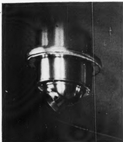
A REVOLVING AND DISTRIBUTING LOUVRE with a concentrated jet, which gives a large radius of effect, whilst rotation ensures that all space within the radius is thoroughly ventilated. Designed and made by Thermotank.
