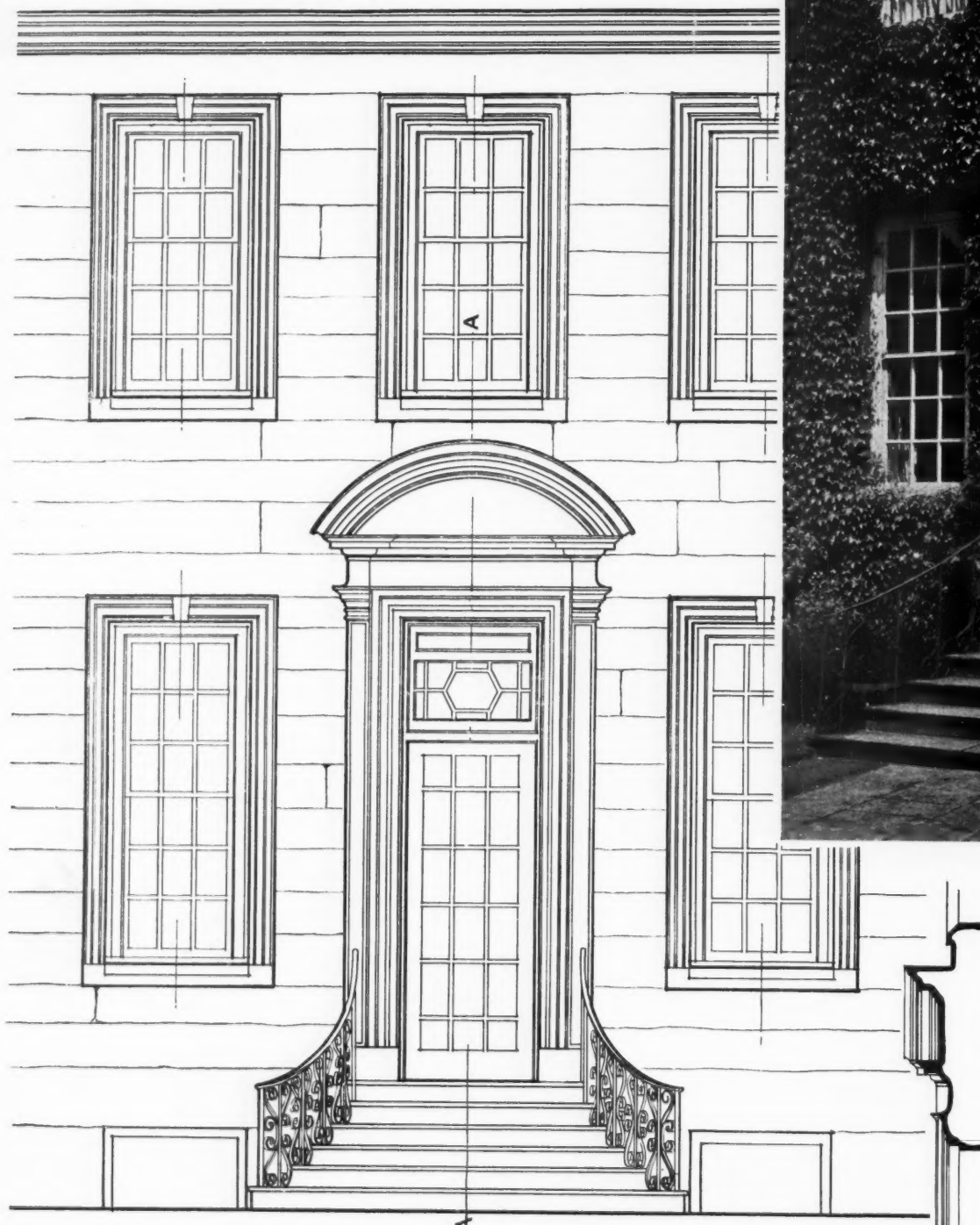
A measured drawing of the elevation, section and plan of the ENTRANCE DOORWAY on the south front of Upton House, near Banbury, Warwickshire. Remodelled by P. Morley Horder.
