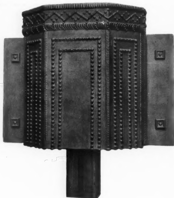
An example of modern Lead-work. All ornaments made on by means of the lead burner.
