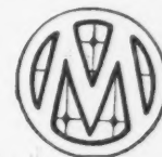
Section of "Eclipse" Patent Glazing Bar.
