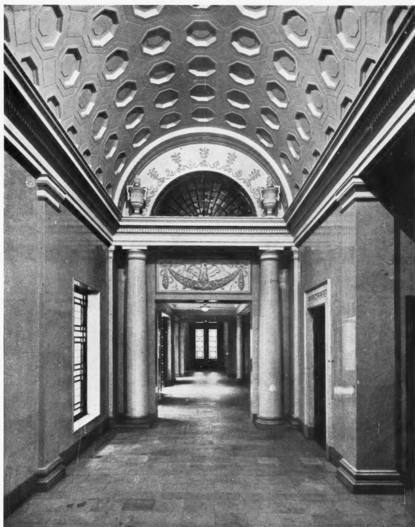
Looking south from the WEST ENTRANCE. The walls and floors are of Subiaco marble and the vault is built of fibrous plaster.
