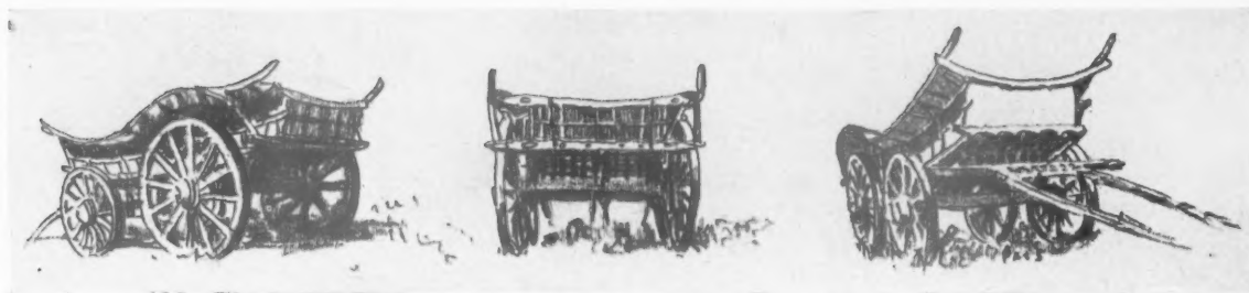
A Gloucestershire type of WAGON for one or two pairs of shafts. It is similar in type to the wagon which Constable was so fond of drawing.
